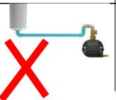
The ½" drain pipe must be horizontal or ideally at a downwards slope (>1°).
